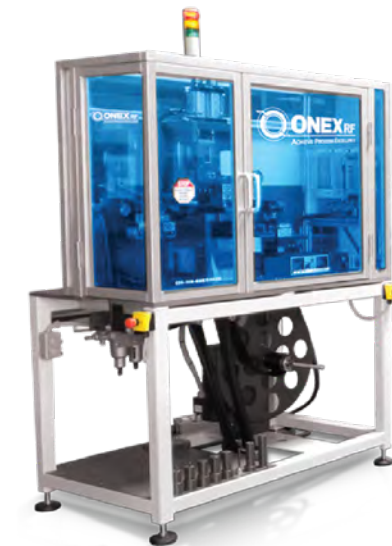
Automated Film Feeder with Punch & Cut Station.
